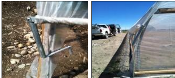
Figure 35 – Hand crank can be locked in position using the structure but is not recommended.
